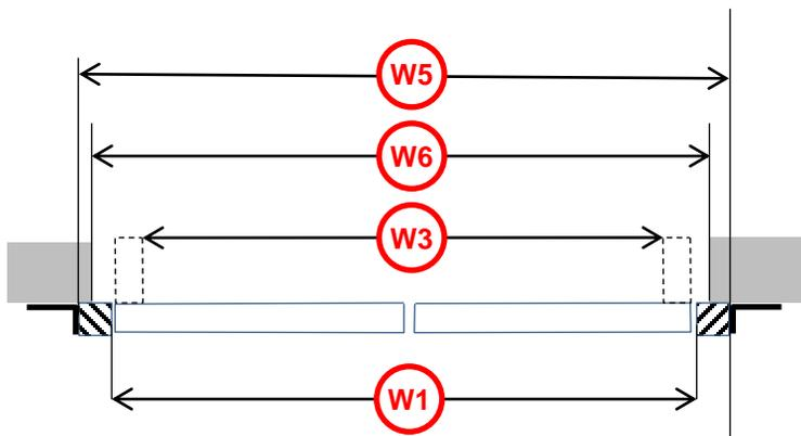
Door Stays to be adjusted to ensure the door panels do not hit the brickwork
